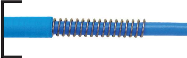
For applications requiring a slightly greater amount of compression resistance (300 lbs/in), but where weight and flexibility are also critical. The cable is covered with a flexible wound helix of passivated stainless steel wire and a cross-linked polyolefin jacket.
