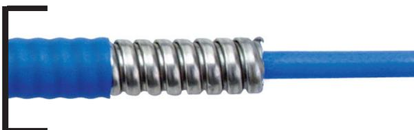
Designed for both inside and outside environments where flexibility and weight are not as critical, but where the application requires the ultimate in cut and crush resistance (500 lbs/in). The cable is covered with a stainless steel interlocked armor; an additional cross-linked polyolefin jacket is standard on lengths up to 50 feet.
