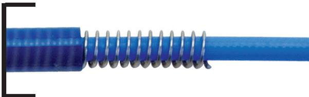
For applications similar to the above, where weight, flexibility, and moderate compression resistance (300 lbs/in) are important, but where abrasion resistance is also critical. The cable is covered with a flexible wound helix of passivated stainless steel wire and an extruded polyurethane jacket.
