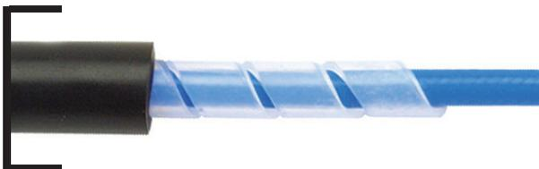
For applications requiring abrasion resistance combined with improved compression resistance (400 lbs/in). Product still remains very flexible. The FEP-jacketed cable is protected with a high density polyethylene anti-compression helix (205 only) that is covered with a tough fuel and oil resistant Neoprene® synthetic rubber. Per MIL-R-6855, Class 2, Grade 60.
